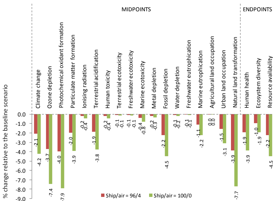
Figure 47: Changes in the life cycle impacts of textiles in the EU-27 resulting from the different transportation scenarios
